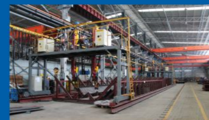
H型钢龙门式自动埋弧焊接机 H type steel Longmen type welding machine
